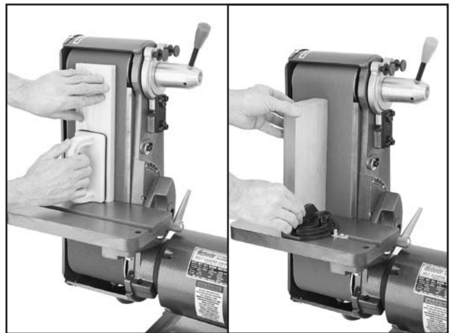
Figure 40. Examples of vertical face and edge sanding.
